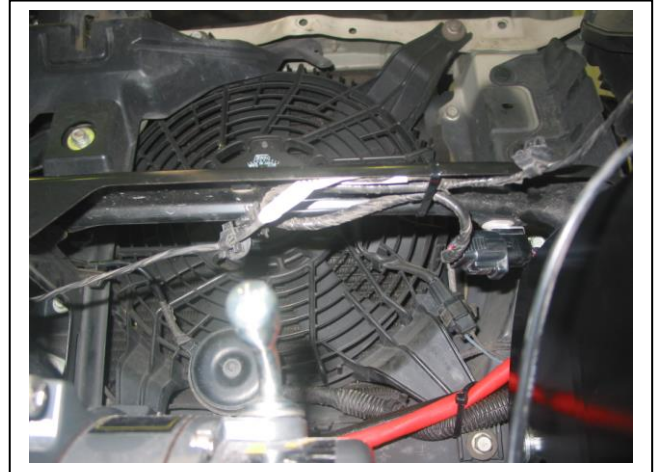
Figure 9: Wiring attached to underside of top bumper support panel.
