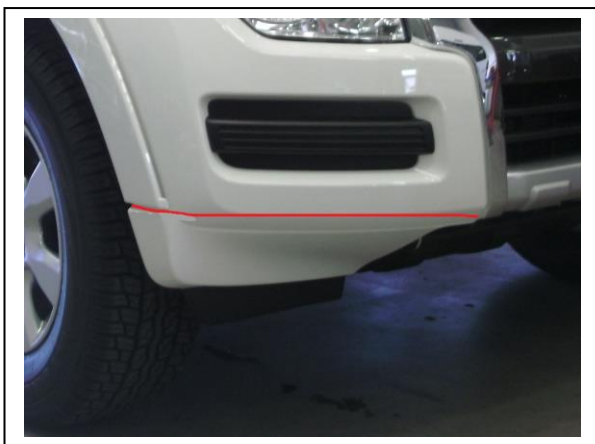
Figure 12: Trim lower section from side of grille opening to bottom of flare on bumper.
