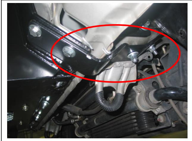
Figure 8: Install lower chassis support. Drill three lower mount holes into chassis rail
